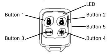
The Astra 777 is supplied with one 5-button Remote Transmitter used to control system operations.
